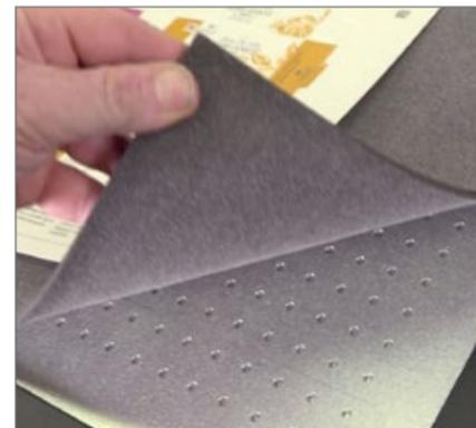
**Vacuum hold down table.** Sheets are held securely in place on either a green self-healing or superior grey felt cutting mat, by a vacuum produced by a powerful centrifugal air pump. Suction passes through the perforated hold down table and the mat, keeping sheets flat and secure.
