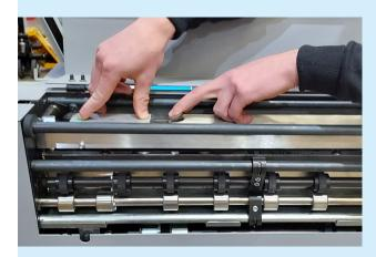
EasyBlade quick release mechanism.
